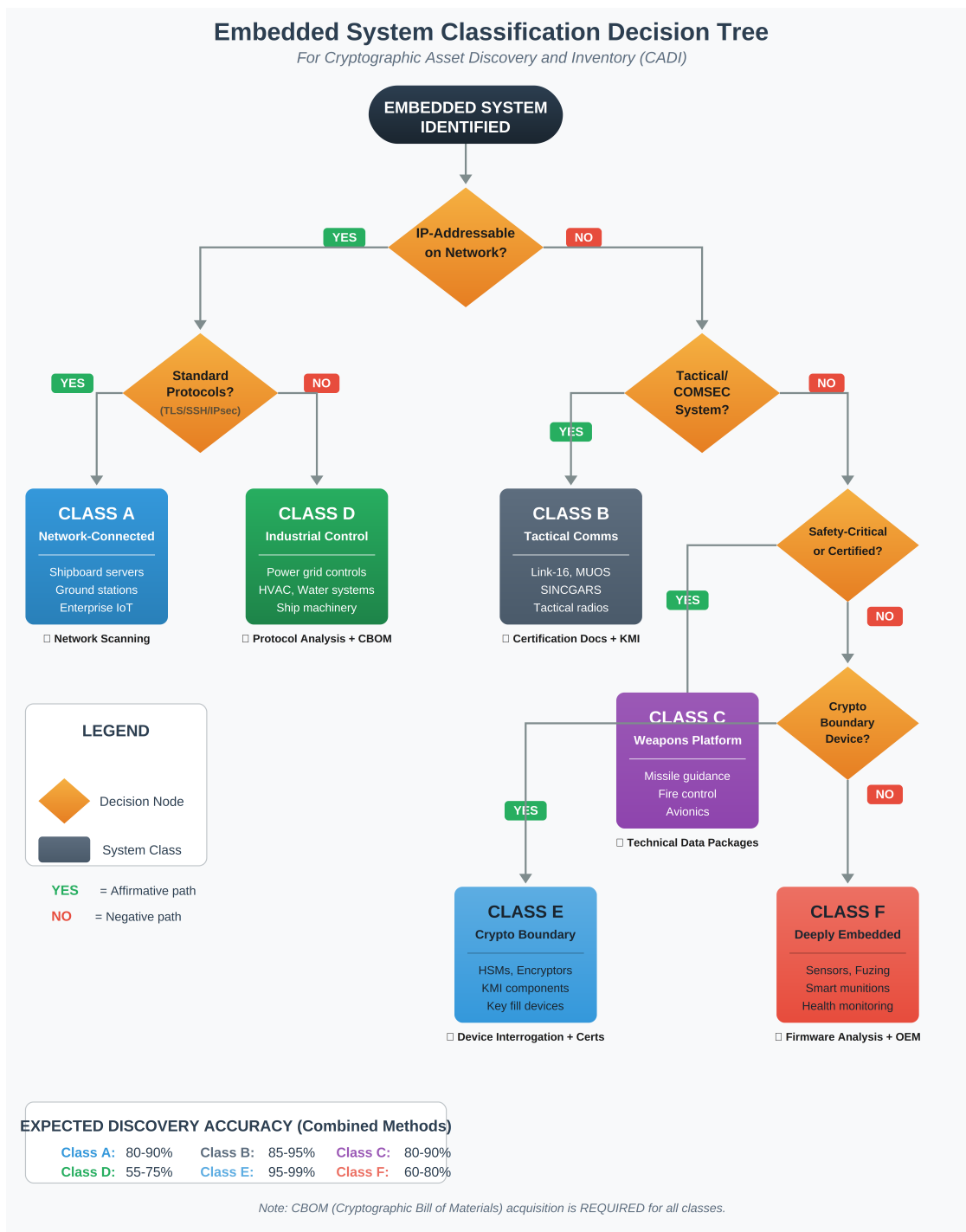
Figure 1. Embedded System Classification Decision Tree for CADI operations.
