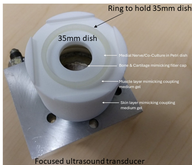
Figure 2. This image shows a custom in-vitro testing fixture designed and fabricated by Mancheung Cheung at the University at Buffalo, USA, for bench-top evaluation of a focused ultrasound transducer system (from Engineering Acoustics Incorporated, USA). The setup features a single-element focused ultrasound transducer mounted on a metallic baseplate for stability and thermal conduction. A white cylindrical holder secures a standard 35 mm petri dish directly above the transducer using a retention ring, ensuring precise alignment of the sample at the transducer's focal distance around 45 mm. The central opening of the fixture with a bone mimicking filler allows the ultrasound beam to pass through coupling medium gel mimicking muscle/skin and focus on the contents of the dish, which may include facet joint capsule/medial branch nerve mimicking phantoms, hydrogels, or co-cultures [14]. This configuration enables controlled testing of acoustic parameters such as peak pressure, cavitation thresholds, thermal effects, and radiation force. It is particularly useful for validating biophysical models like Neuronal Intramembrane Cavitation Excitation under reproducible, phase-zero in-vitro conditions before clinical translation.
