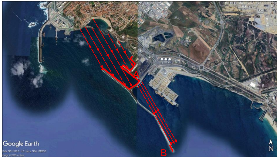
Figure 9. Illustration of fetch length for NWN wind direction and testbed zones A and B next to shore. Adapted from [26].
