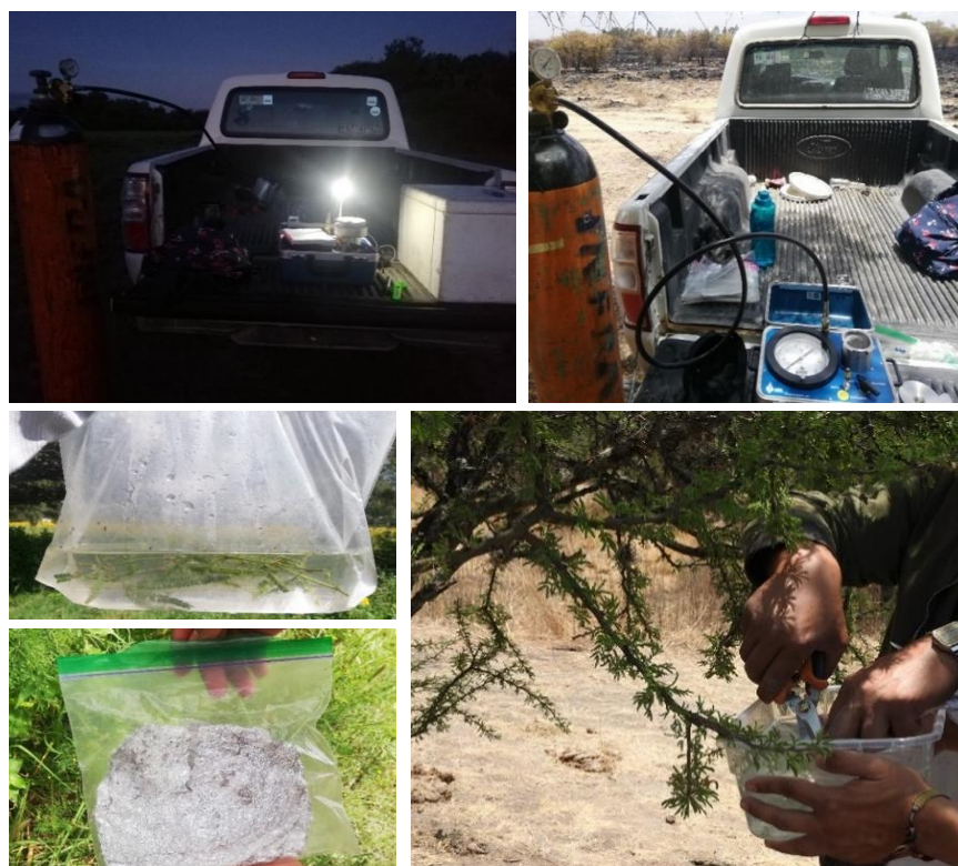
Figure 2. Water potential measurements in field, and sampling of leaves and twigs for making pressure-volume curves in lab.
