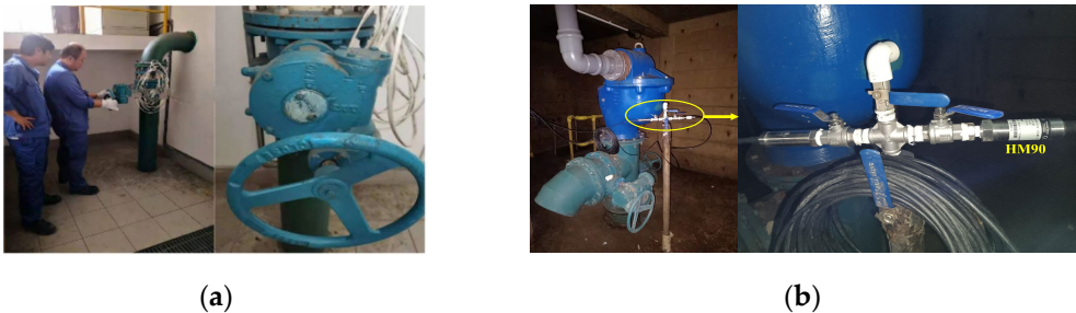
Figure 9. On-site experiment illustrations: (a) Workers' operations with varying valve openings during leak simulation. (b) Pressure sensor installation.
