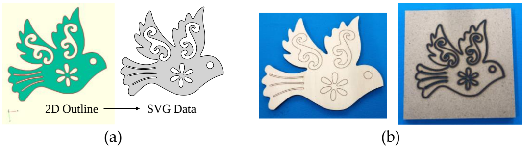
Figure 27. (a) 2D reconstruction and SVG data, and (b) fabricated samples.
