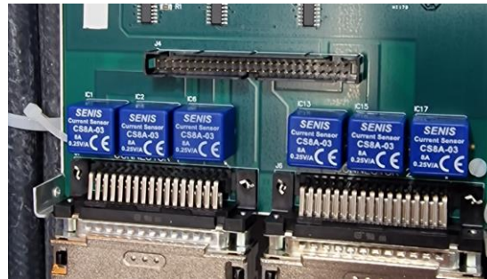
Figure 9. SENIS CS series current sensors applied in the LHCb SciFi detector at CERN for monitoring heating wires.
