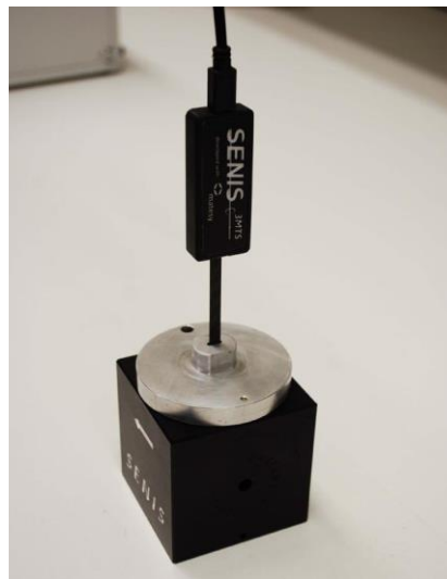
Figure 11. Verification of calibration and orthogonality of the SENIS 3D Hall probe of a SENIS Magnetometer.
