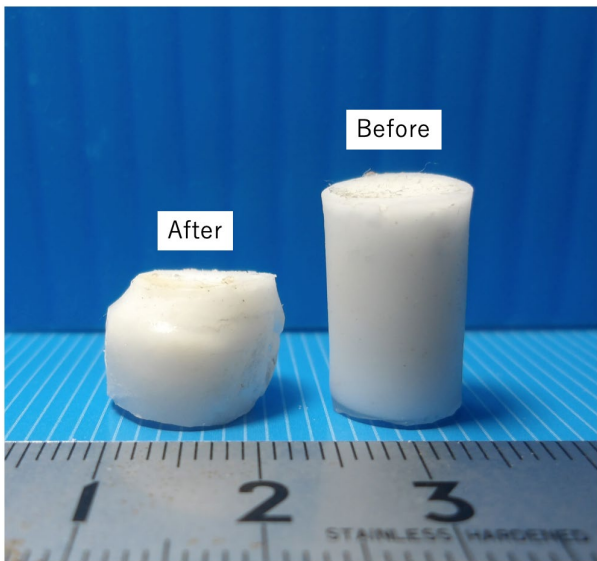
Figure 23. Appearance of BC specimens before and after compression, indicating ductile fracture.
