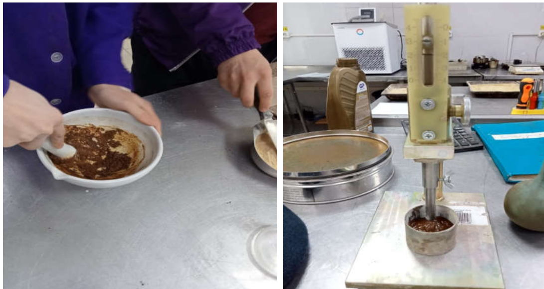
Figure 7. Manual mixing of mineral powder with bitumen and subsequent determination of bitumen capacity using a standardized plunger device
