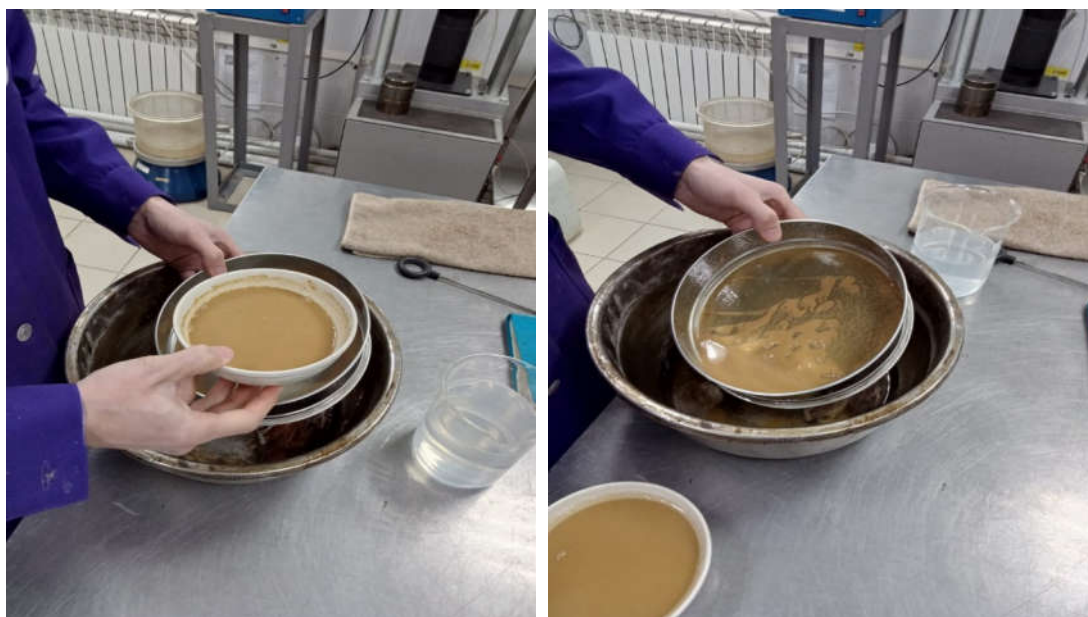
Figure 4. Determination of porosity and particle separation of processed basalt insulation waste.
