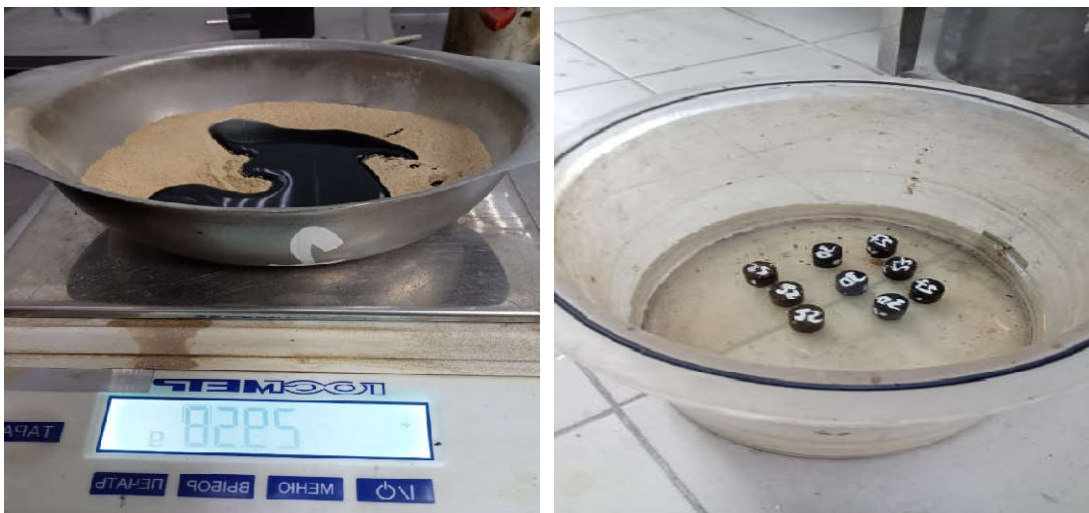
Figure 6. Swelling of samples from the mixture of powder with bitumen
