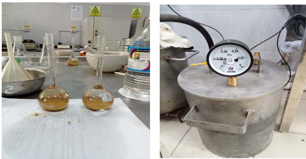
Figure 8. Determination of moisture content of mineral powder
