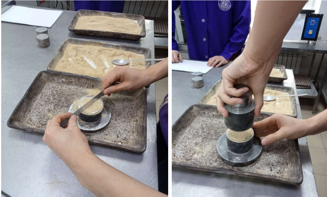
Figure 5. Determination of true density of mineral insulation waste particles using a volumetric compaction device
