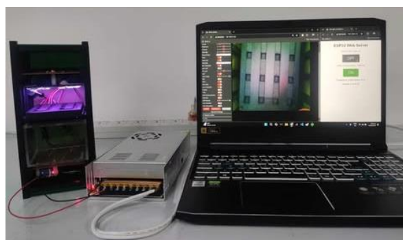
Figure 2. ARCHER (Agricultural CubeSat for Horticulture Experiments and Research) version 1.
