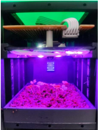
Figure 9. Germinating bed for the ARCHER CubeSat with the ESP32-CAM placed on top and the DHT11 sensor at the back.
