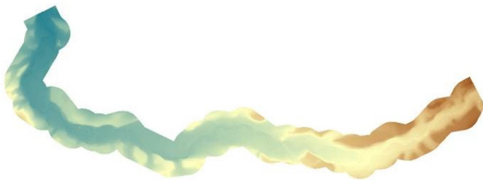
Figure 3. Example for a slope calculation from the PNOA's DTM [40], 1 m pixel size.
