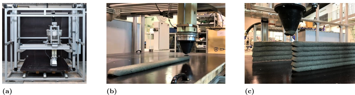
Figure 2: (a) 3D-printer at TU Dresden, (b) extrusion of single layer and (c) multiple layers with a circular, vertical nozzle.
