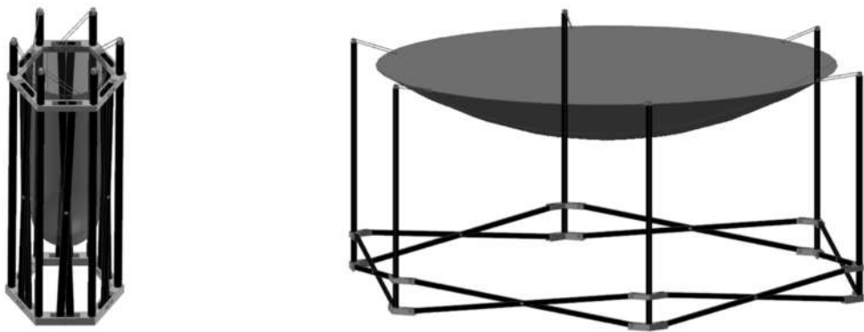
Figure 14. Extendable Truss Deployment Mechanism.
