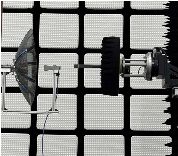
Figure 12. Reflector Antenna in Near-field Test.
