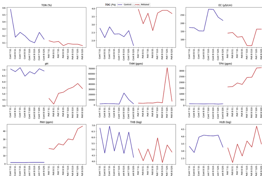
Figure 1. Distribution of the physicochemical and microbiological parameters across the 16 samples. All polluted samples exhibit lower pH than the unpolluted samples, while the control samples have higher pH. The pH of the year 1 polluted samples is lower initially but steadily increases with age. The THM (the sum of the six analysed heavy metals: Cu, Pb, Cd, Fe, Cr, and Ni) concentrations in the control samples do not follow a distinct trend, although surface values are generally higher than those of the subsurface. In contrast, the heavy metal concentrations in the polluted samples increase over time, following a trend similar to that observed for TPH. In summary, spent engine oil reduces soil TON, EC, and pH, but increases TOC, TPH, PAHs, and THMs.
