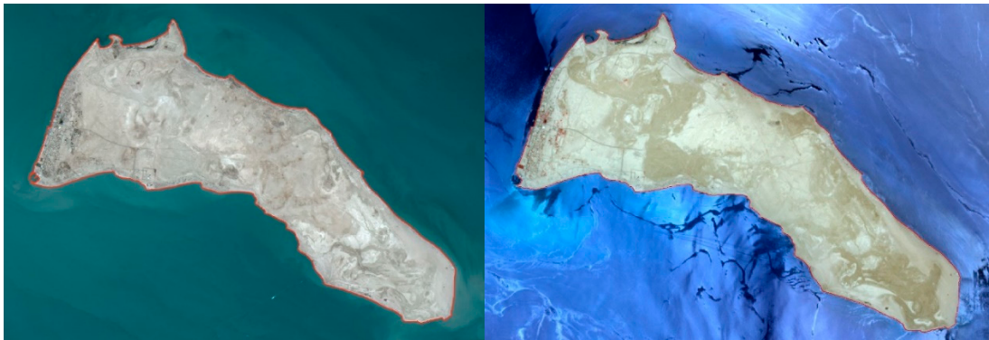
Figure 10. The extracted shoreline with manual analysis of Landsat 8 merged band and Aster VNIR. The images are linear 2%.
