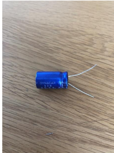
Figure 6. The employed super-condenser. The capacitance is 3.3 F, and the standard voltage is 2.5 V.
