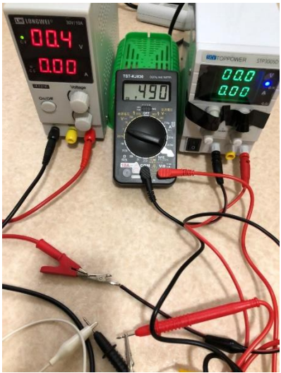
Figure 7. The right-hand power supply changes from the cc mode to the cv mode, and the voltage of the super-condenser was charged to approximately 0.49 V. Notably, when the right power supply changes from the cc mode to the cv mode, its voltage is 0.0V. This implies that the input of the voltage to the cc mode of the current source is zero. For details, see the main body in this paper.
