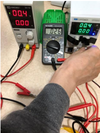
Figure 7. A current from the cc mode of the current source is supplied to the system.
