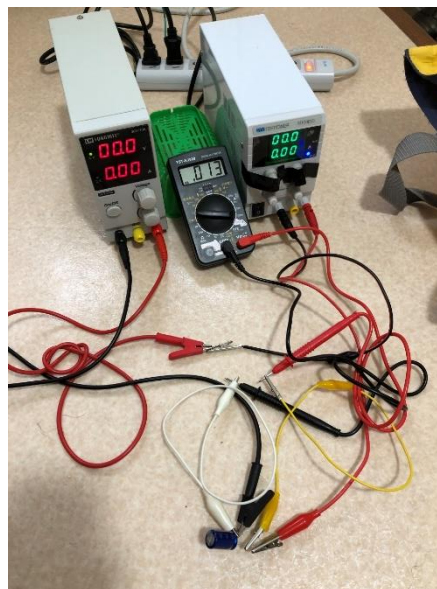
Figure 7. The complete view of the system. In this figure, the left stabilized power supply (i.e., red character) is a cv mode, and the center device is a voltmeter for the super-condenser, and the right stabilized power supply (i.e., green character) is a cc mode. Notably, the super-condenser is blue and located below.
