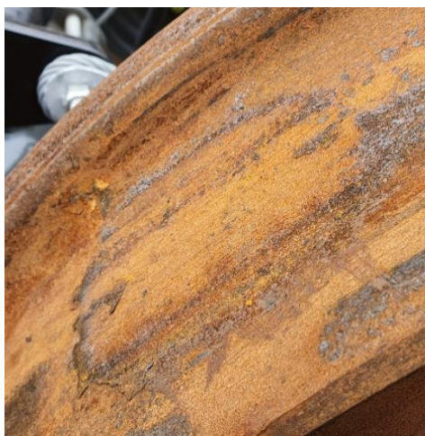
Figure 1. Flat spots—caused by blocking of the wheel set by the axle box seizure.
