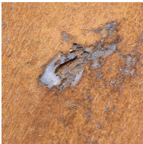
Figure 2. Chipping—defects that occur on the running surface of the wheel, these are holes created by the detachment of the wheel's native material.
