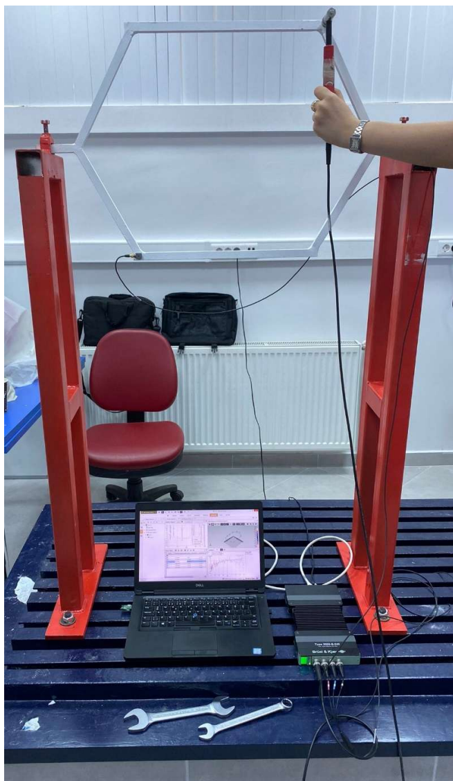
Figure 28. The experimental setup of a hexagonal test piece.
