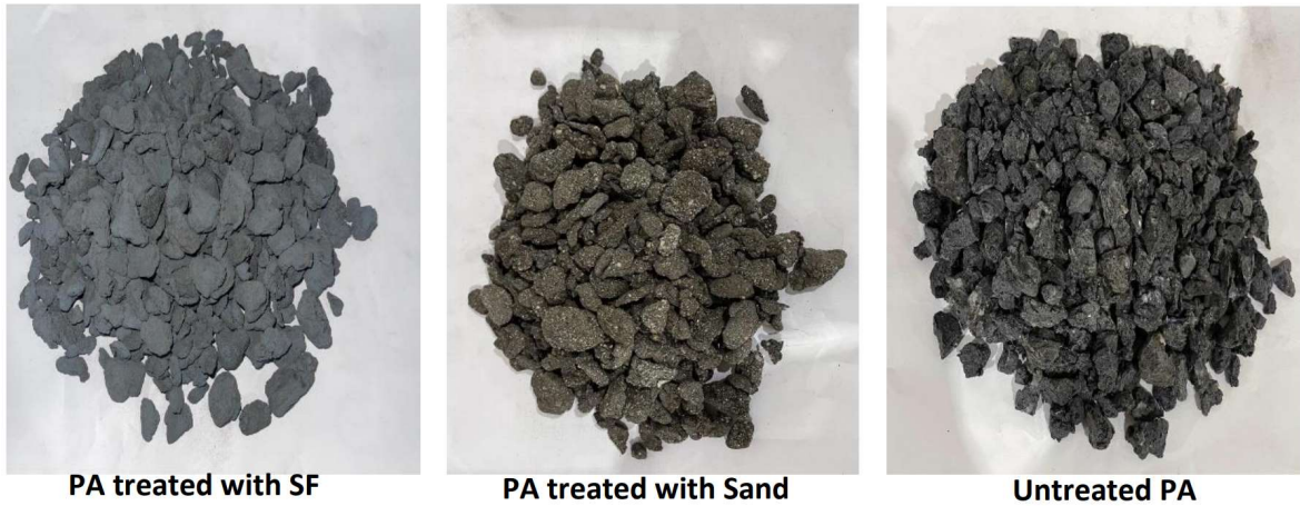
Figure 2. Shapes of treated and untreated plastic aggregates.
