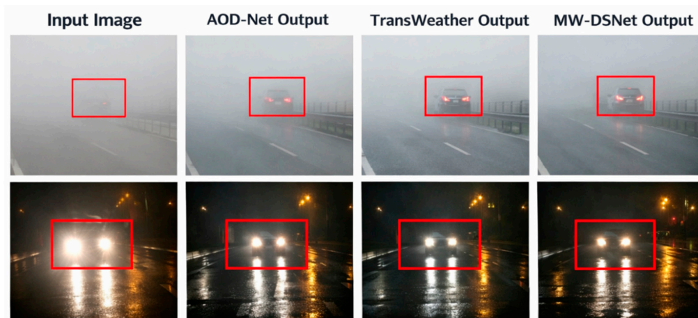
Figure 8. Qualitative comparison of visual restoration results under dense fog and night-glare conditions. Columns show the degraded input, AOD-Net, FFA-Net, TransWeather, and the proposed MW-DSNet. Red boxes highlight safety-critical areas of interest, including distant vehicle boundaries, lane markings, and structures adjacent to intense headlights. MW-DSNet more effectively suppresses glare-related blooming and preserves fine structural details.
