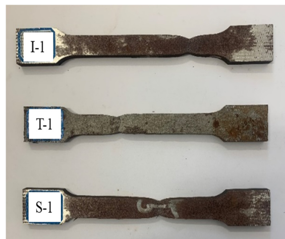
Figure 5. Tensile test ruptured specimen.
