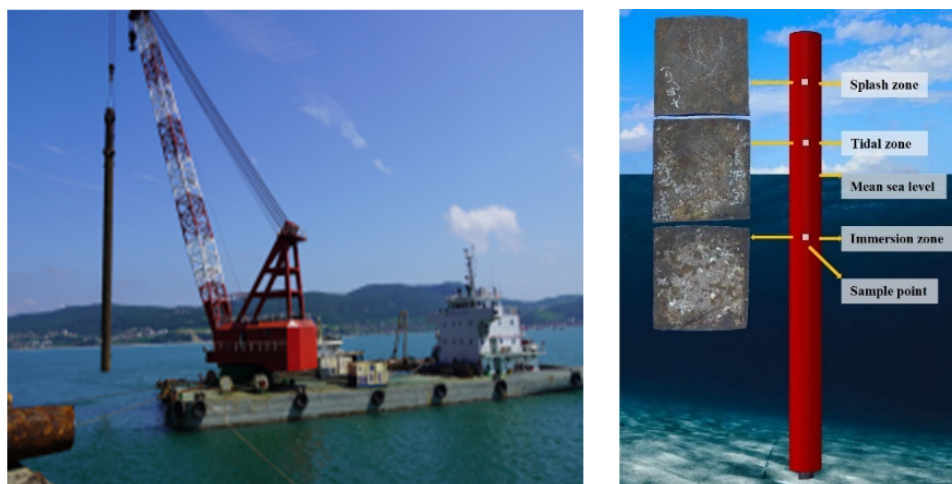
Figure 2. Steel pipe pile and specimen locations.
