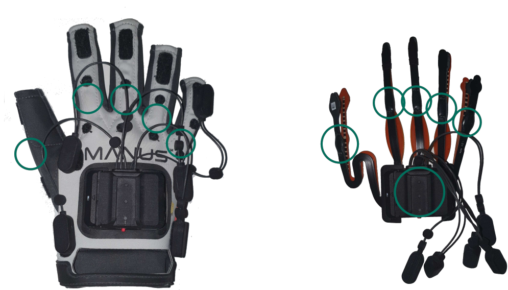
(a) Green circles indicates the IMUs. (b) Brown strips indicates the flex sensors.
