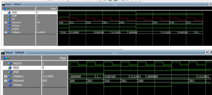
Figure 13. Hardware Trojan Simulation in ModelSim.
