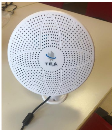
Figure 2. AirQino Indoor LITE monitoring station.
