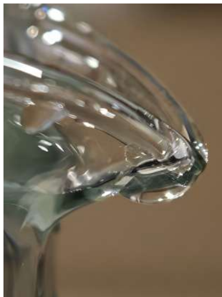
Figure 7. Spout model exhibiting the teapot effect in a glass teapot.
