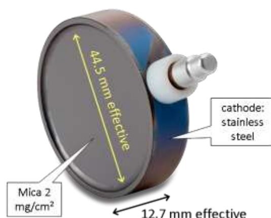
Figure 2. LND 7317 Pancake GM detector. Picture from the manufacturer's web page.
