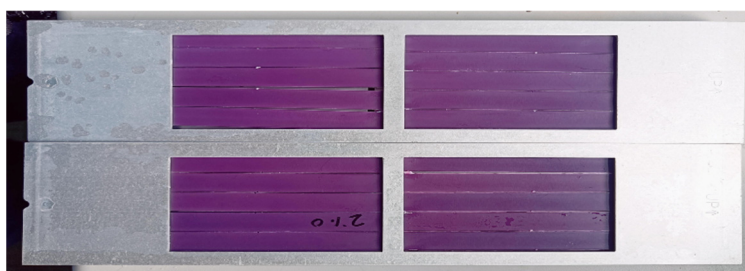
Figure 5. Samples mounted in metal frames prior to accelerated aging in the QUV weathering chamber.
