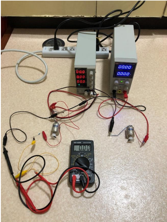
Figure 10-2. Initial setup of the experiment for harvesting the current I_E' . Shown are the two voltage sources, the paired motors, a current meter (range 10 A), and a 1.0-MΩ resistor connected by the red and yellow leads (in the vicinity of the left motor).
