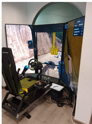
Figure 2. The simulator in action, integrating motion, visuals, and controls with real-time performance tracking.
