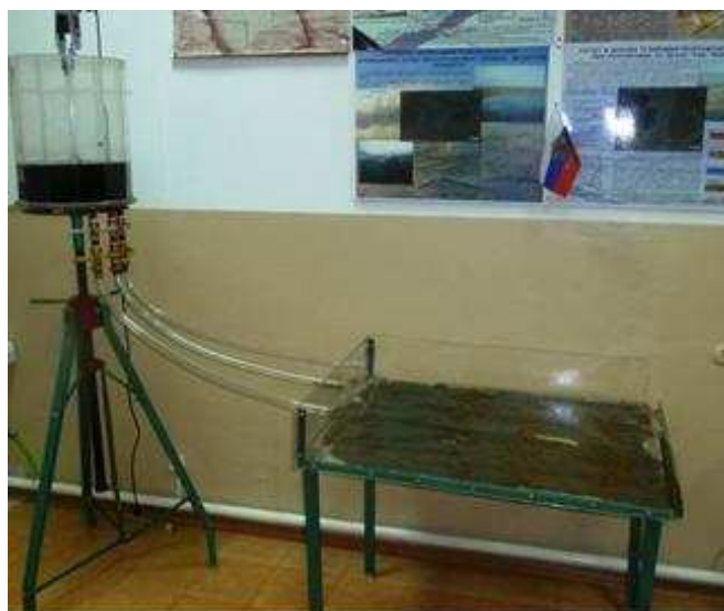
Figure 9. The design of a laboratory setup for modeling the alluvium of the tailings dam.
