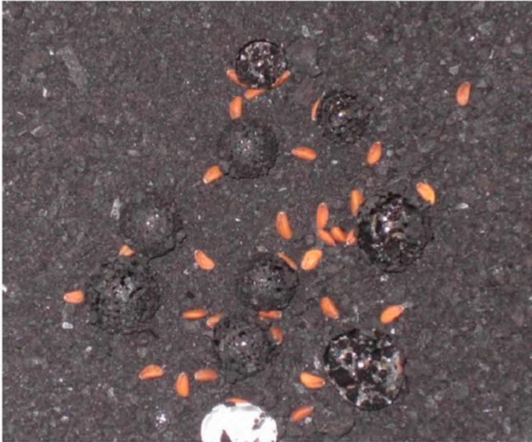
Figure 27. Bubbles of water on the surface of TOR 350 demonstrating char hydrophobicity.
