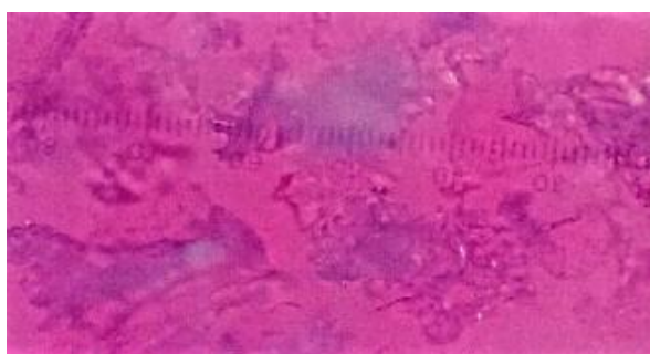
Figure 2. Microscopic form of pregelatinized cornstarch with magnificant 100 times.
