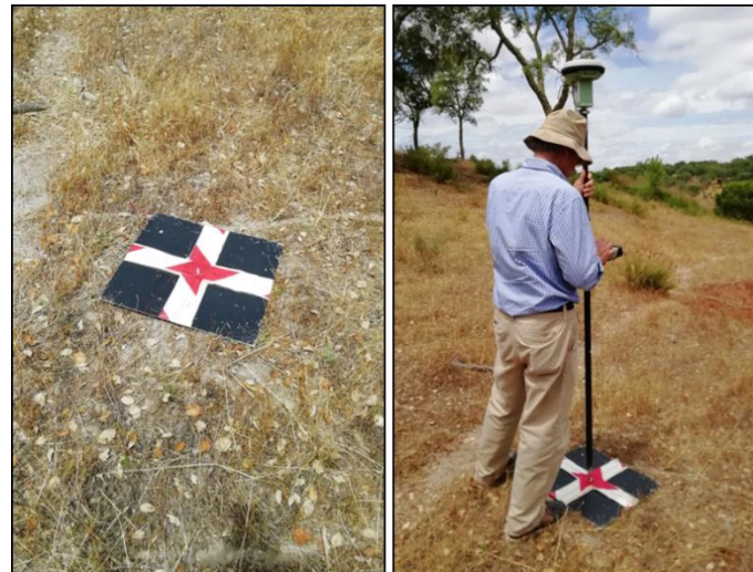
Figure 3. In-situ photos of GCP used to rectify the UAV imagery.
