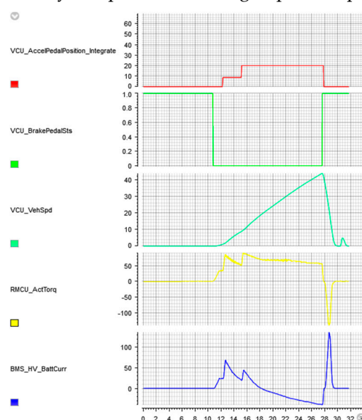
Figure 11. Key signal timing diagram of driving and braking conditions.
