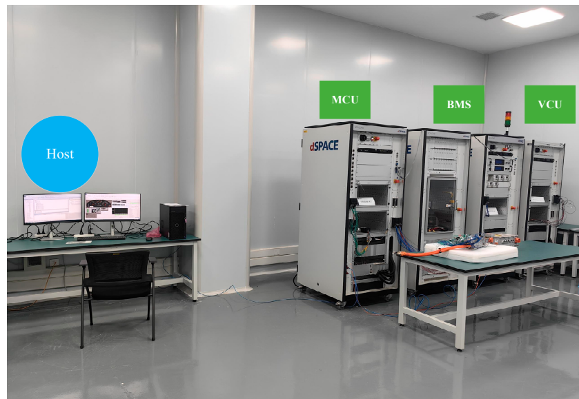
Figure 8. The physical drawing of the powertrain digital twin bench.
