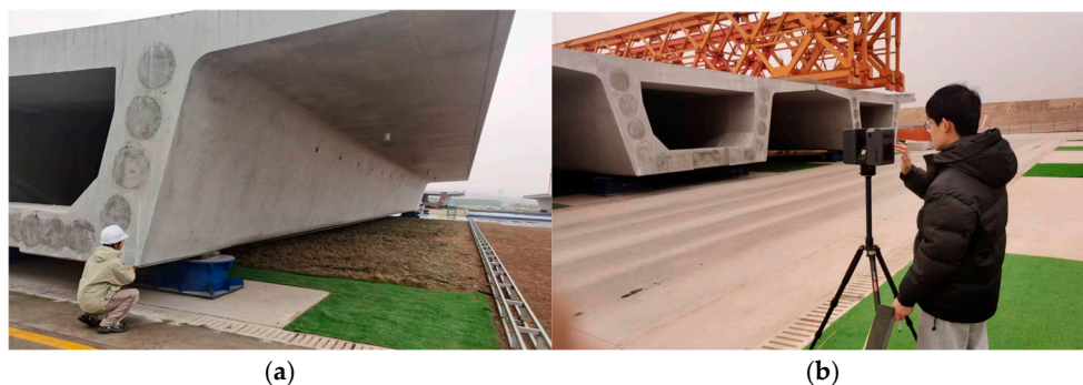
Figure 15. Comparison of Detection Processes:(a) Manual Measurement Monitoring;(b) 3D Laser Scanning Monitoring.
