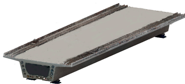
Figure 10. Complete Box Girder Point Cloud Model.
