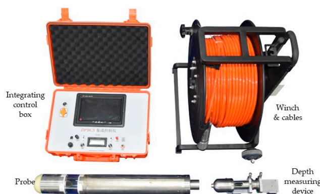
Figure 3. The basic components of a typical borehole digital optical camera system.
