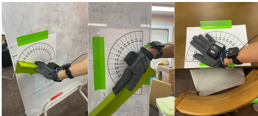
Figure 5. Verifying the accuracy of the motion-capture glove's orientation.
