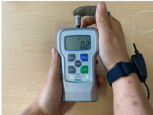
Figure 6. Experimental setup for sensor calibration using a force gauge and the finger-mounted sensor.
