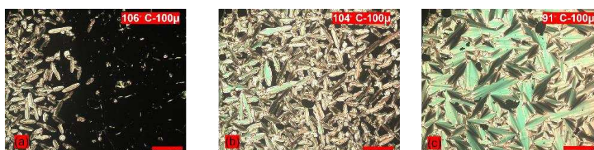
Figure 13. Optical polarization microscopy of mixture of M1: MCN ; molar ratio = 1.2: 0.8. The scale bar is 105μm. (a) phase transition from a nematic phase with a homeotropic orientation to the SmA phase at 106°C (b) SmA phase at 104°C (c) SmA phase at 91°C.
