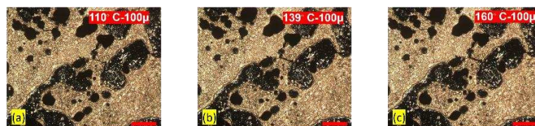
Figure 11. Defec texture of homopolymer 1 ( HP1 ), as by optical polarization microscopy. The scale bar is 105 \mu\text{m} (a) at 110 °C (b) at 139 °C (c) at 160 °C.
