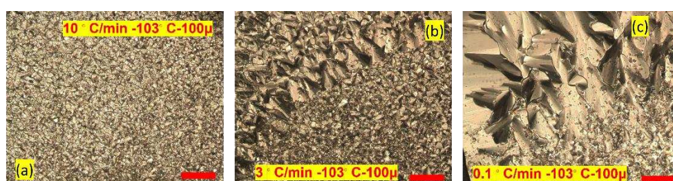
Figure 5. Textures measured by OPM of M1 at the 103 °C at different cooling rates. Top left is the N tb phase, and bottom right is the nematic phase. (a) cooling rate at 10 °C/min under 103 °C (b) cooling rate at 3 °C/min under 103 °C (c) cooling rate at 0.1 °C/min, under 103 °C.
