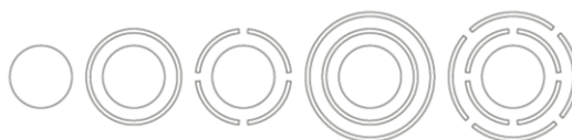
Figure 3. Schematic design of the four predetermined breaking structures surrounding the inlets in comparison to the usual inlet (left). A more detailed version is given in SI Figure S3.
