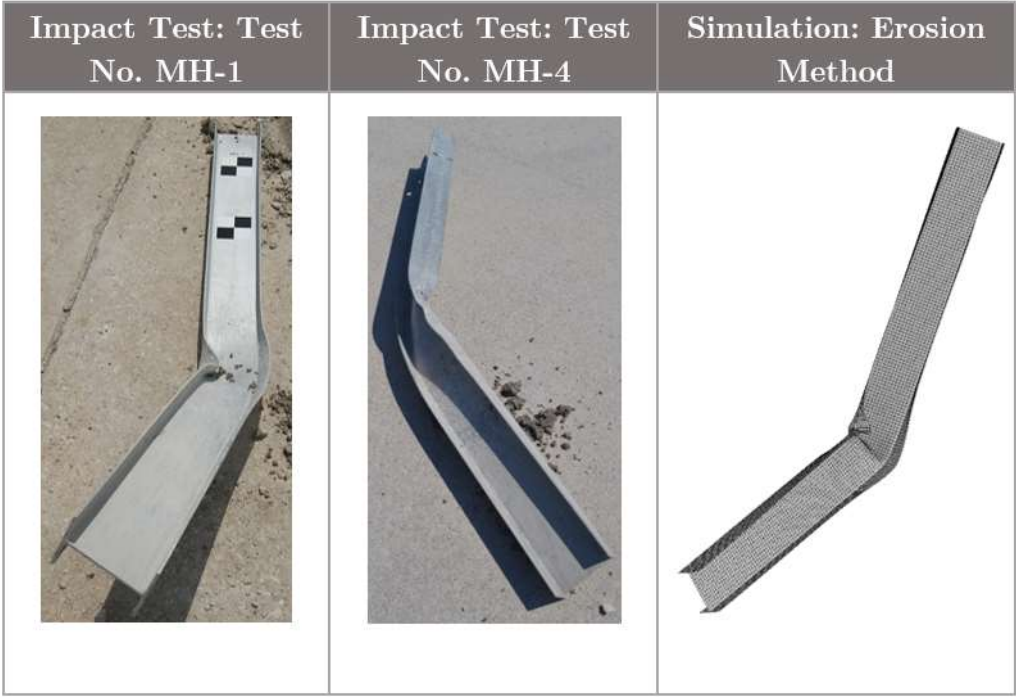
Figure 4. Post-impact photographs of buckled W152x12.6 steel pile, physical impact test and simulation using erosion method.
