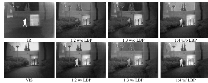
Figure 10. Ablation experiment on TNO dataset. From left to right: source images and fusion results of LPGAN with different settings.
