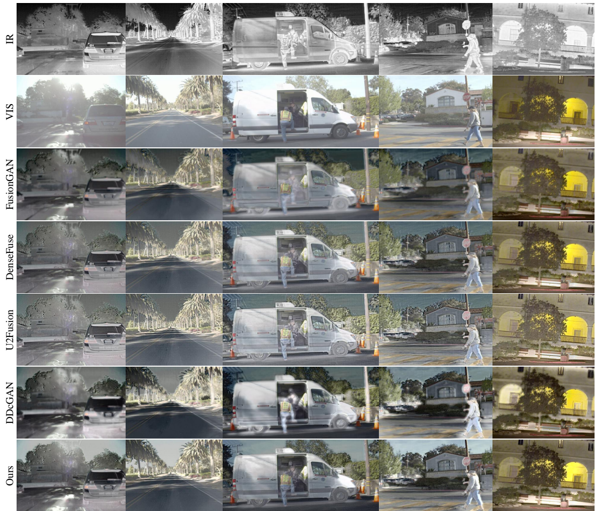
Figure 12. Fused results on the 5 image pairs in the RoadScene dataset. From top to bottom: the infrared images, the RGB images and the fused images.
