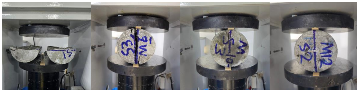
Figure 11. Failure mode of 0%, 0.2%, 0.8% and 1.4% WSRF for plain concrete.
