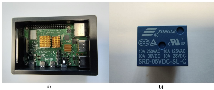
Figure 6. a) Raspberry Pi 4 Model-B 8GB RAM. b) Relay module. 5V DC SRD-5VDC-SL-C.
