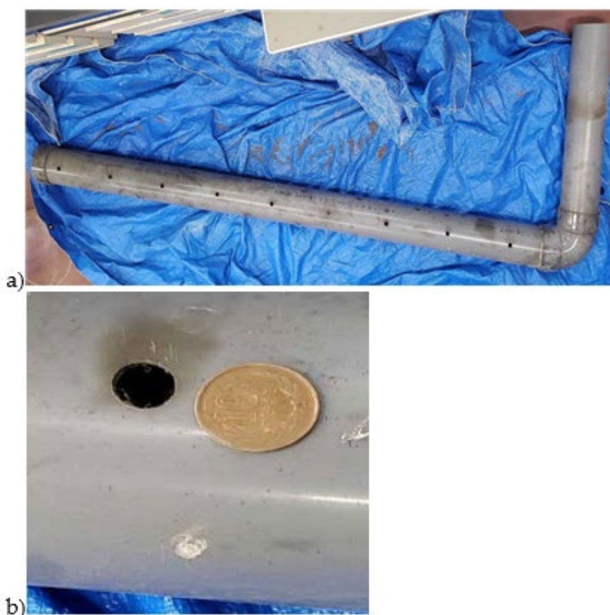
Figure 1. Buried PVC pipe for MNB application: (a) Overall view: (b) a 12 mm diameter hole drilled so that the MNB exits the PVC pipe. The 10 yen coin placed next to it is 32 mm in diameter.
