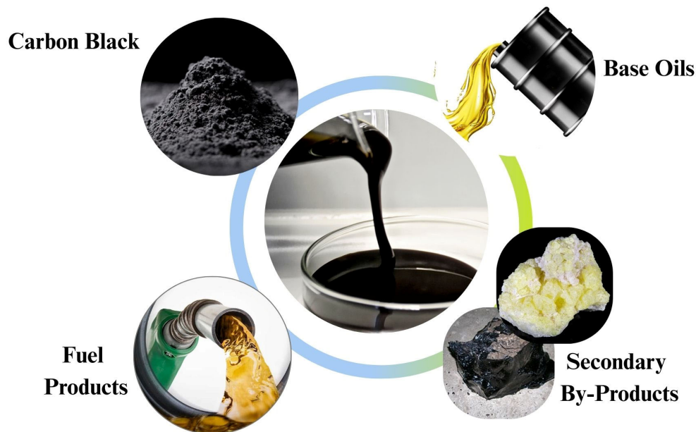
Figure 9. Valuable petrochemical products and carbon-based materials obtained from waste lubricating oils (WLOs).
