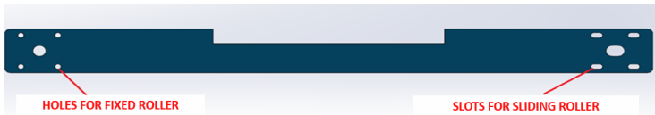
Figure 16. Side face 1 of the metal structure
