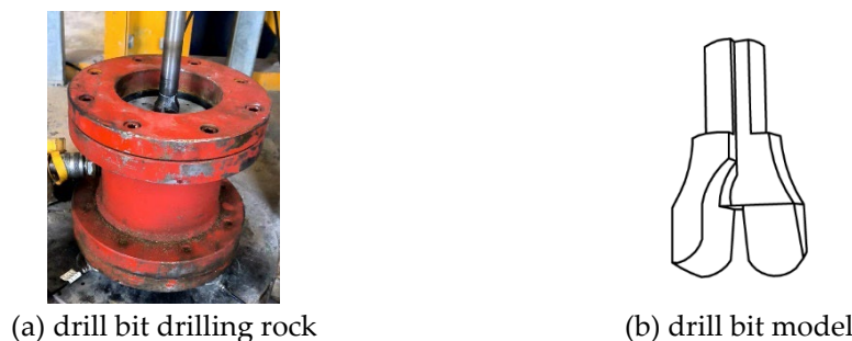
Figure 2. Double-wing PDC bit.
