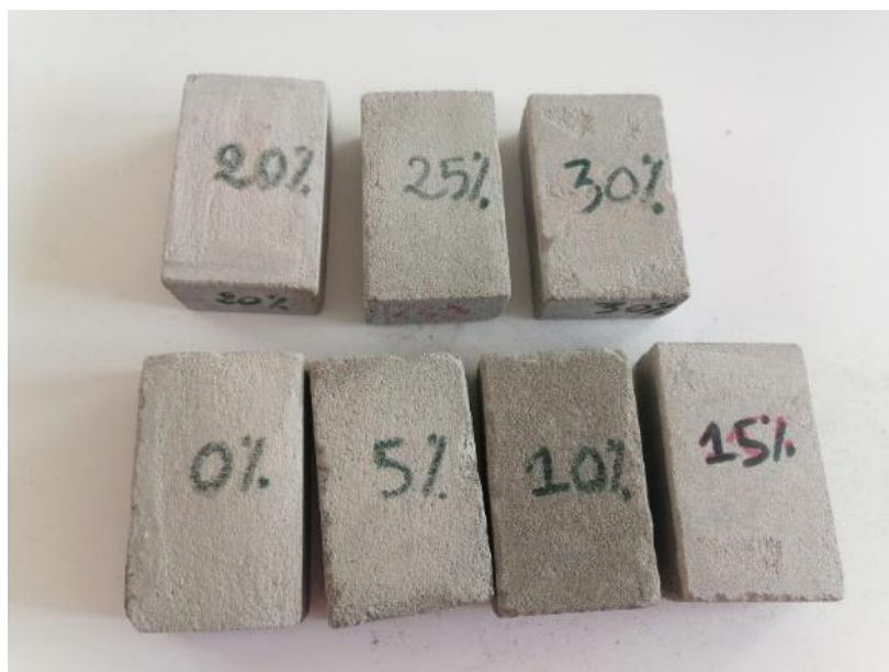
Figure 2. Mortar samples for thermal conductivity measurements.
