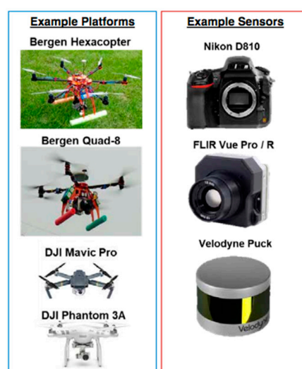
Figure 8. Examples of MTRI UAS drone options: Bergen Hexacopter and Quad-8, assorted small (sUAS) quadcopters (e.g. DJI Mavic Pro, DJI Phantom 3A). Example sensors carried by drone platforms are shown in right panel.
