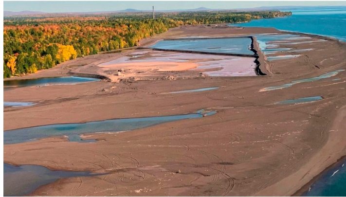
Figure 14. Drone photo of “Berm Complex” (2021), in the stamp sand Pond Field southwest of Gay (stack site), berm walls were constructed from local stamp sand. Plastic pipes carried in dredged stamp sands from the Traverse River Harbor and “Trough”. The darker reddish-brown sediments are stamp sands in the Pond Field beach, whereas the lighter pink and orange sediments are recently deposited dredged spoils within the berm walls (2020-2021). Notice water percolating through berm walls into bordering ponds. The outer shoreline thickening is also part of a “revetment-like” stamp sand addition, intended to protect the Berm Complex from enhanced shoreline erosion. (photo by MDNR).
