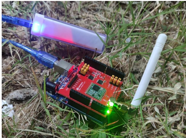
Figure 6. Terminal device: Arduino Uno + LoRa Shield and power bank power supply.
